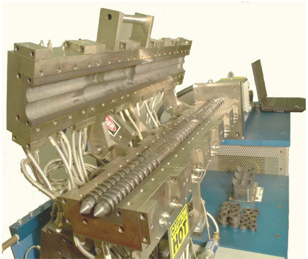
Example of counter-rotating intermeshing screw configuration
